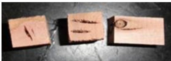
Figure 1. Specimens with node, collapse, and low extractive deposition.
